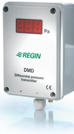
**DMD is a differential pressure transmitter for air and neutral gases. The unit has LED-display and built-in controlling function. The main application is for pressure control in air handling systems.**
